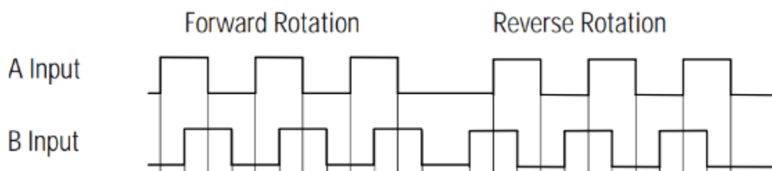
Figure 4: DC motor encoder A and encoder B states for rotation.
